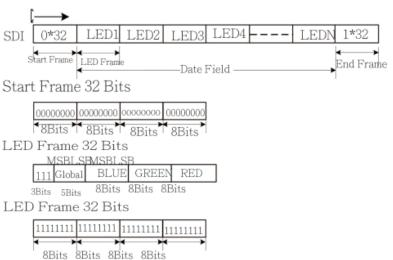
Global bit: 5-bit ( 32 level ) brightness setting, while controlling R, G, B three-color constant current output value, if set the Global bit for the 10000 ( 16/31) is the output current is half again the original PWM settings.
